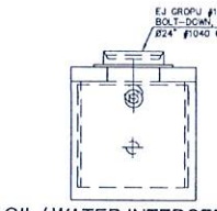
OIL / WATER INTERCEPTOR END VIEW
